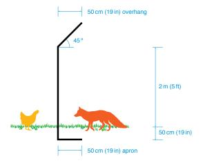
**Fox-proof fencing:** This is a plan for non-electrified fences to prevent foxes from getting into poultry pens. An alternative is to bury the apron wire at a 45-degree angle, rather than at the 90-degree angle shown above, or pave around the perimeter with the mesh running under the slabs. You can eliminate the need for an overhang and increase the security of the run by covering the top with mesh, completely enclosing the pen. Illustration not to scale.
