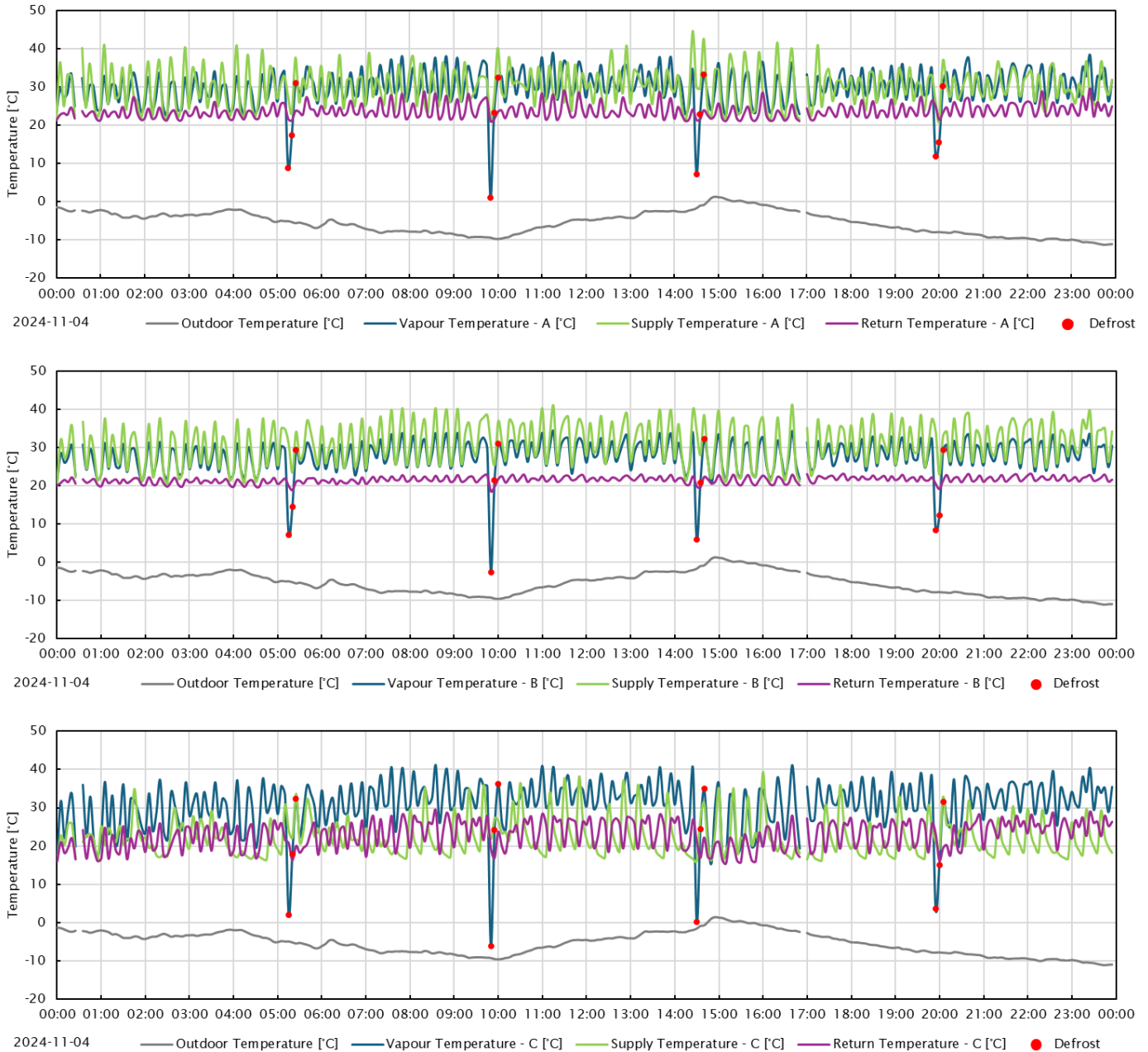
Figure 3.4 Heat pump cycles for site WH-03 (ductless system with 3 indoor units), during a sample day on November 4, 2024. Each indoor unit has its own subplot. The blue, purple and green lines show the vapour line, return airflow, and supply airflow temperatures of the heat pump, respectively. The grey line shows the measured ambient outdoor temperature. Data points that are considered part of the defrost cycle are shown in red.
